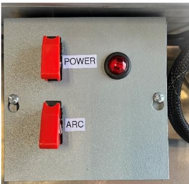
**Press the control button to activate the UTV torch.**
